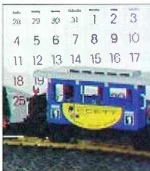
Figure 2. Line replication involves doubling field 1's lines, then repeating field 2's lines, etc. Note the "blockiness" created on the numbers and the "jaggies" present on the train's yellow semicircle.
