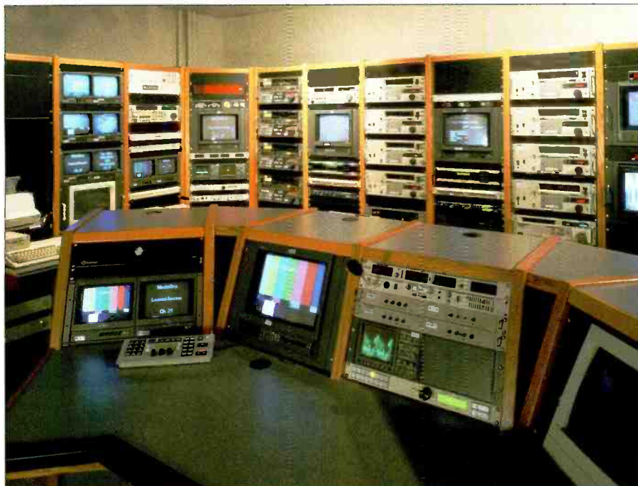
Master control console. L-R logo inserter control and monitoring, network monitoring, router control and logging computer display.
