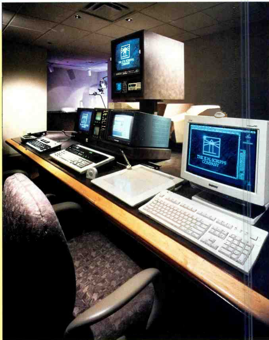
Graphics room No. 3 uses SGI computers, iNFiNiT! workstations and Macintosh computers.
