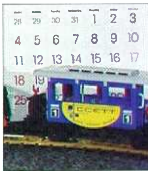
Figure 3. Vertical and temporal filtering — images are cleaned up substantially. This is the method Genesis Microchip uses, and motion video will appear cleaner and more stable.
