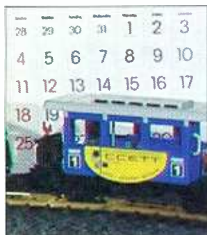
Figure 1. The field merging process involves slapping together two fields to produce a video frame. Notice the "squiggly" motion artifacts on the calendar numbers. This would look bad running at 30fps.
